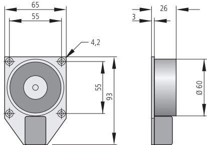
**Flexibler Anker/Induit flexible/flexible doorplate AFS 65**
